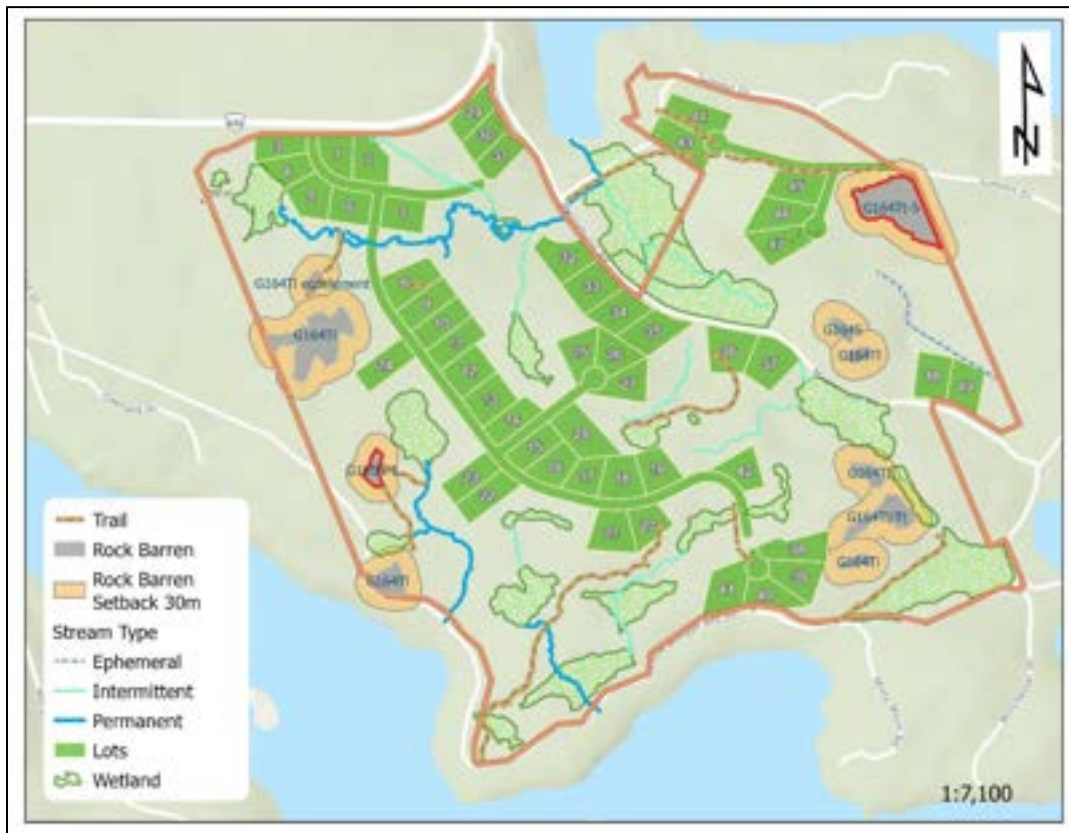
Figure 154: Recommended 30 metre rock barren setbacks; note the two exceptions are highlighted in red outline where existing access and trails are permitted to continue. The watercourses and wetland units are shown for reference (without their respective setbacks).
