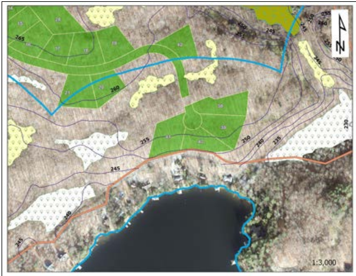
Figure 152: Five metre (5m) contours representing the elevation above sea level; note Lake Rosseau is less than 240 masl while the proposed lots 38 – 41 are 250 – 255 masl. The presence of hardwood swamp wetlands to the north of proposed lots 38 – 41 confirm the land slopes to a lower elevation before rising to 260 masl further north.
